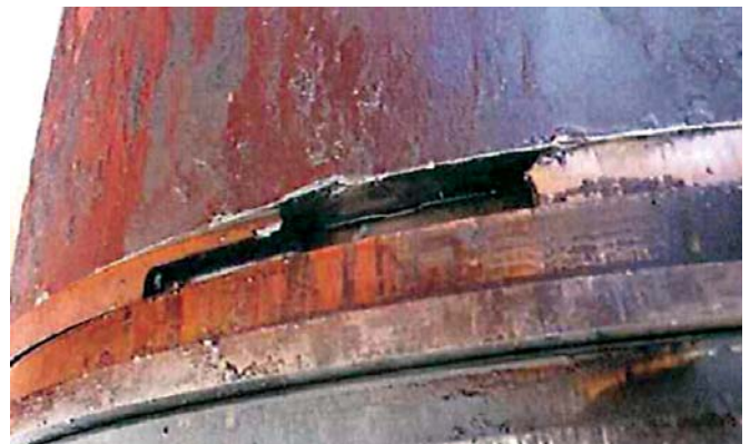
Figure 1 Abrasive wear of piston ring.
