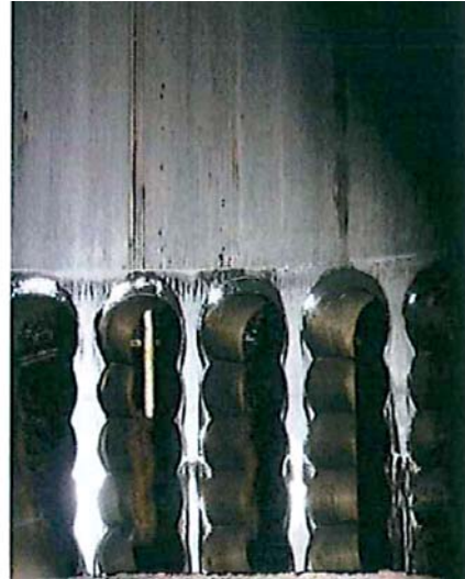
Figure 5 Abrasive wear inside the cylinder liner above the scavenge air ports.
