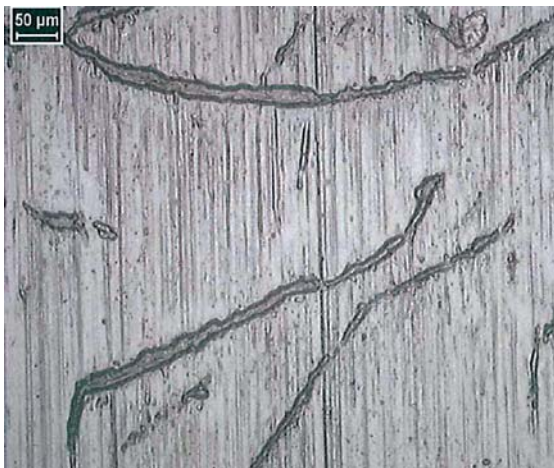
Figure 2 Micrograph (200x magnification) of a normal liner surface with open graphite structure. Dark areas are showing the graphite lamellae.
